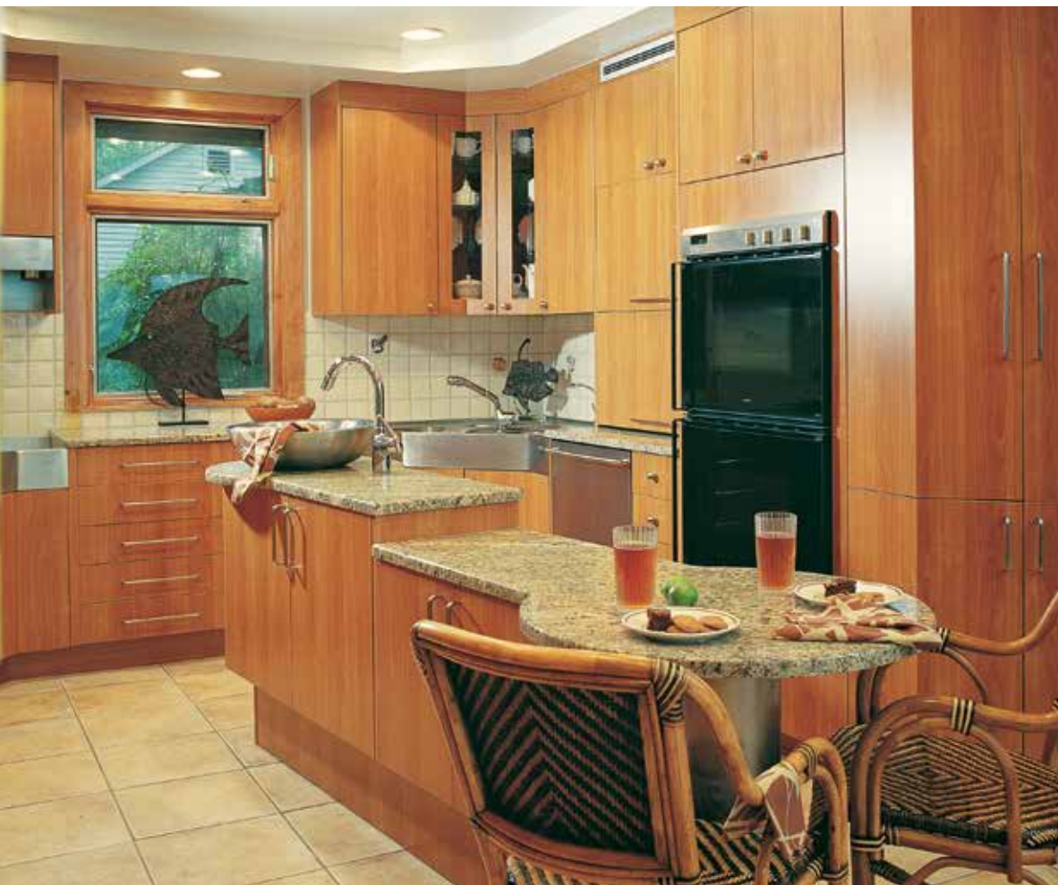
LEFT AND OPPOSITE While many universal kitchen designs include extrawide aisles for wheelchairs, here the aisles have been narrowed to support the home owner, who has difficulty moving about the kitchen or standing for long periods of time. Also, the island is slightly angled to be near to the side-opening ovens in order to make it easier and safer to remove hot pots and pans. Corner-placed appliances, together with a vessel sink on the island, augment the functionality of this beautiful kitchen. Design: Mark T. White
